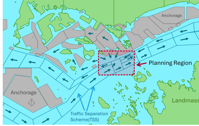
Figure 2: The red region is used as the environment area. The gray areas indicate anchorage zones, the green areas represent landmasses, and the arrows and regions with dark blue borders represent the Maritime Traffic Separation Scheme (TSS). The high density of crossing points in the red area makes it a more challenging region for navigation, providing a suitable setting for testing advanced planning techniques.
