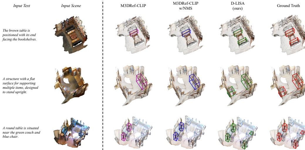
Figure A1: Additional qualitative examples of Multi3DRefer val set in MT category. For each scene-text pair, we visualize the predictions of M3DRef-CLIP, M3DRef-CLIP w/NMS, D-LISA and ground truth labels in magenta/blue/green/red separately.
