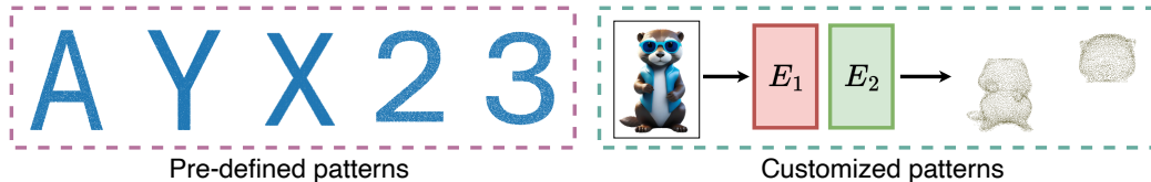
Figure 3: Two different target geometry patterns. (1) Pre-defined patterns: we directly convert alphanumeric characters into a 2D point cloud as watermarks. (2) Customized patterns: In E_1 , we first extract the point cloud of the image that needs to be protected. In E_2 , we edit the acquired point cloud through text-guided methods like instructP2P [48] or open-source software meshlab [5].
