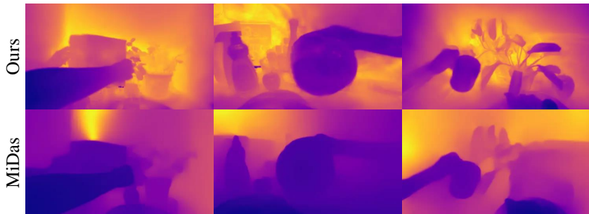
Figure 10: Rendered depth from 3D Gaussian splatting (ours) and off-the-shelf monocular depth estimator (MiDas). Our rendered depth has richer details and is scale-aligned with the scene. MiDas rendered depth is usually more smooth and suffers from scale ambiguity.
