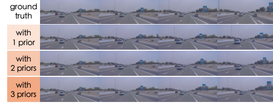
Figure 11: Effect of dynamic priors. Injecting more dynamic priors yields more consistent future motions with the ground truth, such as the motions of the white vehicle and the billboard on the left.
