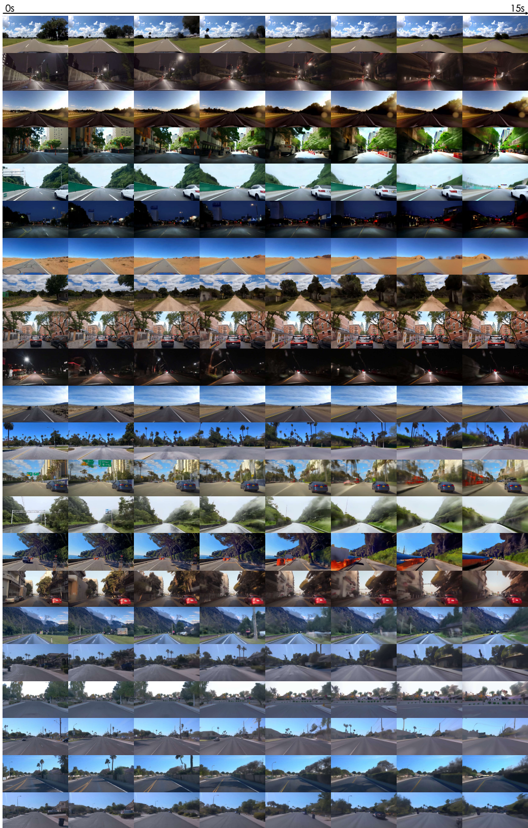
Figure 20: Additional results of long-horizon prediction. Our model can autoregressively simulate long driving experiences with marginal quality decline. All videos continue for 15 seconds at 10 Hz.
