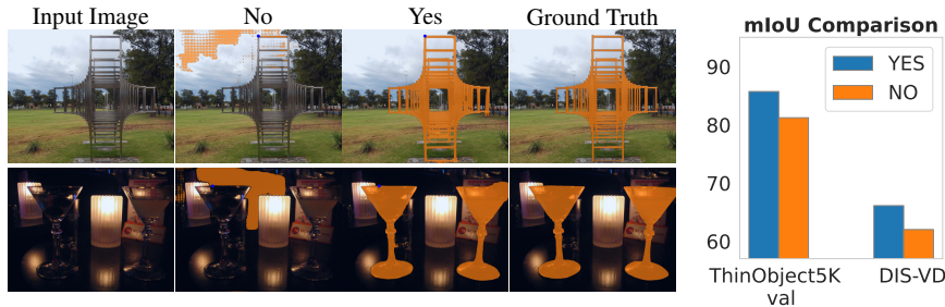
Figure 13: Comparison of SUM and a version of SUM without uncertainty-aware sampling on intricate structures when the prompts are close to object boundaries. In such cases, uncertainty-aware sampling provides visually superior results (left) and a higher single-prompt mean IoU comparison on two challenging test sets (right).
