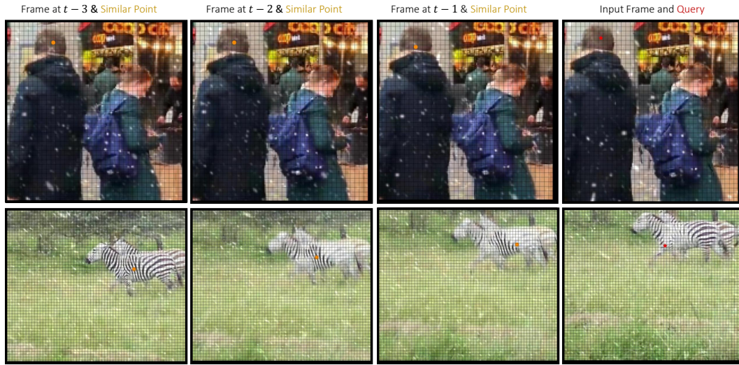
Figure 7: CHM Tracking. Visual illustration of CHM tracking query points in the frame history (frames previous to the input frame). In the top row, we plot the correctly tracked points , while the bottom row visualizes the limitations in the case of redundant patterns. We plot the query and most similar points on input frames for ease of exposition, but in practice, they function on feature maps.
