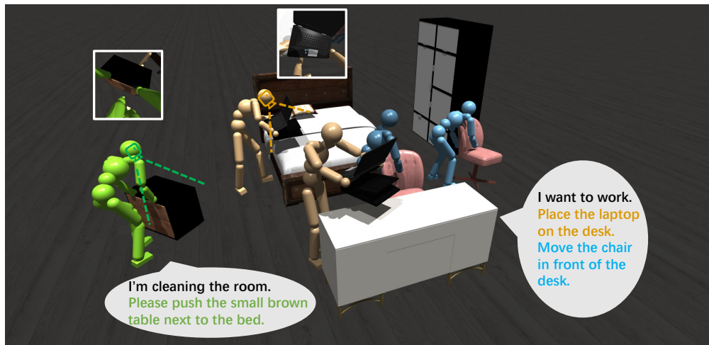
Figure 1: HumanVLA performs various object rearrangement tasks directed by the egocentric vision and natural language instructions.
