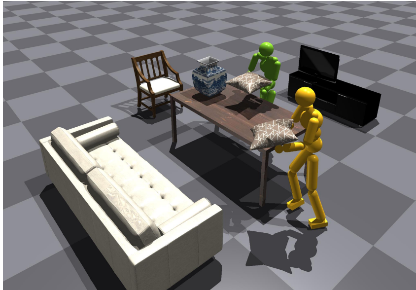
Figure 11: Comparison w/ and w/o path planning. The green humanoid without path guidance fails to get close to the sofa, while the yellow humanoid with path guidance learns to go around the central table. Instruction: Move the pillow to the sofa.
