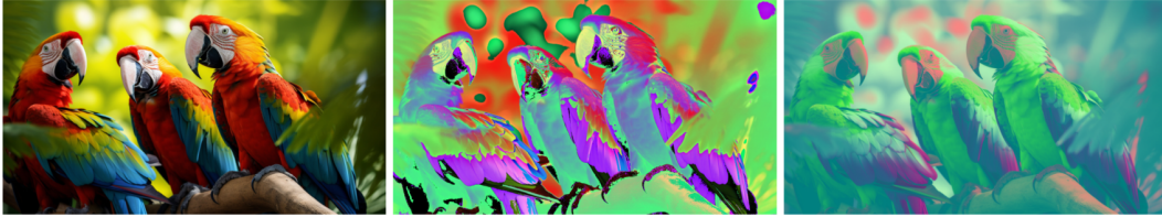
Figure C.4: Visual difference of YCoCg-R and YCoCg. Given the RGB image to the left, we show the application of YCoCg-R in the middle and that of YCoCg to the right.
