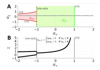
Figure S6: A) Analytically calculated stability regions for a 2-cycle  $\mathcal{S}_{\mathcal{RL}}$  (red), and a fixed point  $\mathcal{S}_{\mathcal{R}}$  (green) for the 1d skew tent map, as defined in the figure, in the parameter plane given by  $(a_r, a_l)$ . B) Bifurcation diagram along the cross section indicated by the gray line in A, showing a BCB and DFB occurring simultaneously at  $a_r = -1$  and a DTB occurring at  $a_r = 1$ .
