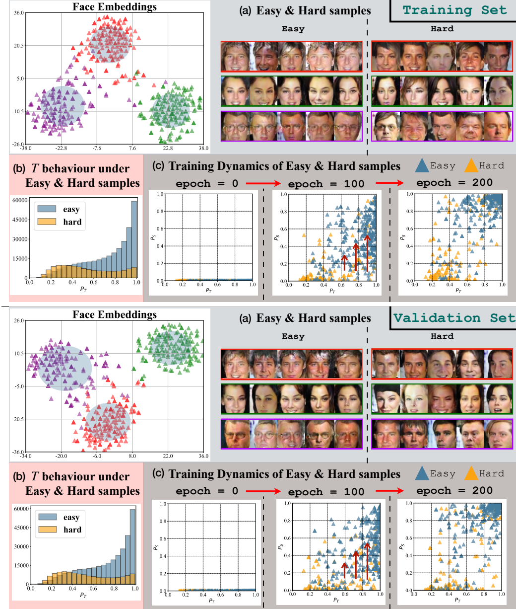
Figure A.6: We use \mathcal{D}_{priv} = \text{CelebA} [3], \mathcal{D}_{pub} = \text{CelebA} [3], T = \text{FaceNet64} , S = \text{DenseNet-161} . The face embeddings are extracted using publicly available SOTA face recognition models here. Similar to our main paper, we apply the framework of [2] to analyze learning dynamics of S to reason why S possesses P1 , and therefore could be an effective proxy for T under MI. We analyze generated samples x_f from our T-ACGAN for 3 identities (IDs 121, 95, 163). We use 150 samples for each identity and show results for both the training set (top) and the validation set (bottom). Note that x_f analysis is relevant as generated samples are used in MI attacks. (a) : Different clusters and different distances from cluster centroids can be observed, suggesting patterns of face identities in some samples (easy samples) while diverse appearance in other samples (hard samples). We use distances from centroids to identify easy samples x_f^e and hard samples x_f^h (easy samples are indicated using a transparent blue circle for each ID in the visualization). Visualization of x_f^e and x_f^h in image space further demonstrates identity patterns in x_f^e and diverse appearance in x_f^h . (b) : Similar to [2], we observe that x_f^e and x_f^h tend to have high and low likelihood under T ( P_T ) resp. This is shown using 500k training data (top) and 500k validation data (bottom). (c) : We track likelihood under S ( P_S ) for x_f^e and x_f^h during the training of S . As training progresses, P_S of x_f^e and x_f^h improve in general, and samples move up vertically (note that P_T of samples do not change). Consistent with the “DNNs Learn Patterns First” finding in [2], S learns general identity patterns first to fit the easy samples. Therefore, P_S of x_f^e improve at a faster pace in the training, and many of them achieve high P_S at epoch = 200. As x_f^e tend to have high P_T , we observe property P1 in S . For x_f^h (many of them tend to have low P_T ), it is uncommon for S to achieve high likelihood on them as they do not fit easily to the pattern learned by S . Best viewed in color.
