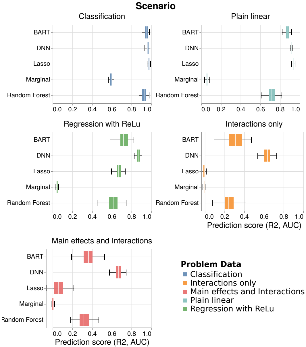
Figure 6: Evaluating predictive power: Performance of the different base learners used in the variable importance methods ( Marginal = {Marginal effects}, Lasso = {Knockoff-Lasso}, Random Forest = {MDI, d0CRT, CPI-RF, Conditional-RF, cpi-knockoff, LOCO}, BART = {Knockoff-BART, BART} and DNN = {Knockoff-Deep, Perffit-DNN, CPI-DNN, Lazy VI}) on simulated data with n = 1000 and p = 50 in terms of ROC-AUC score for the classification and R2 score for the regression.
