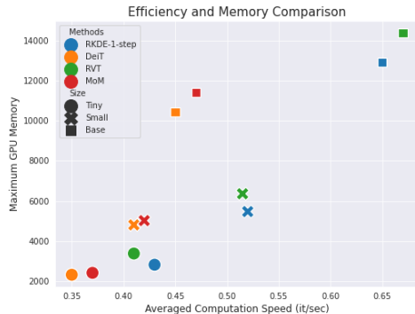
Figure 4: Comparison of averaged computation speed (measured by iteration per second) and maximum GPU memory (measured by the CUDA max_memory_allocated function) on ImageNet classification task. The results are measured under the Transformer base models with different capacities: Tiny ( 5.7M parameters), Small ( 22M ), and Base ( 86M ).
