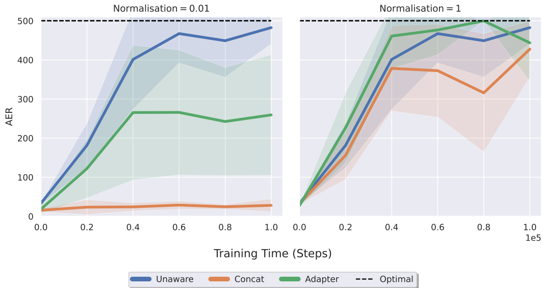
Figure 27: Performance when evaluating on changing Pole Mass when normalising with respect to (left) Mass = 0.01 and (right) Mass = 1.0. In both plots, the models trained on Mass = 0.01. Mean performance is shown, with standard deviation shaded.
