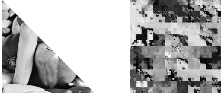
Figure 19: An example of the encoding map taking data from a triangular domain and mapping it to an array of each 'triangular pixel' value under lexicographical ordering.
