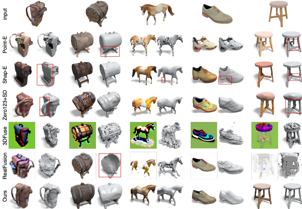
Figure 6: We compare One-2-3-45 with Point-E [57], Shap-E [30], Zero123 (Stable Dreamfusion version) [41], 3DFuse [72], and RealFusion [48]. In each example, we present both the textured and textureless meshes. As 3DFuse [72] and RealFusion [48] do not natively support the export of textured meshes, we showcase the results of volume rendering instead.
