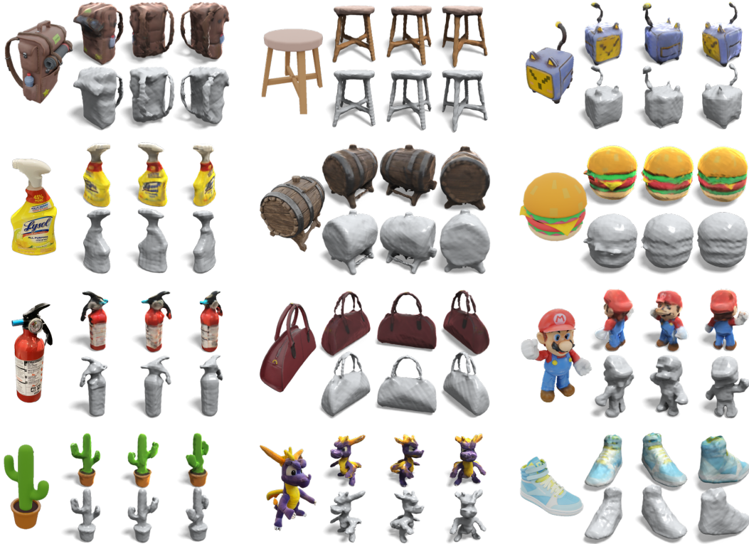
Figure 1: One-2-3-45 reconstructs a full 360° mesh of any object in 45 seconds given a single image of it. In each example, we showcase the input image in the left column, alongside the generated textured and textureless meshes from three different views.
