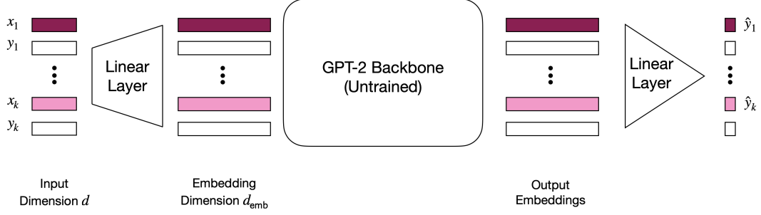
Figure 15: TART reasoning module architecture. The reasoning module takes as input sequences of (x, y) pairs of dimension d . A linear layer is used to project d to the hidden dimension size of the GPT-2 backbone. Finally, a linear layer is applied to the outputs of the backbone to generate predictions for each x_k in the input sequence.
