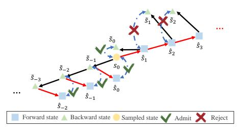
Figure 2: Illustration of the double check mechanism in bidirectional modeling. We use the trained opposite dynamics model to check whether the synthetic transitions generated by the current dynamics model are reliable. We are confident about the transitions that can be traced back to the starting state with small errors (green check) and reject those with large disagreements (red cross).
