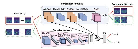
Figure 2: Overview of DyAd applied to two inputs of fluid turbulence, one with small external forces and one with larger external forces. The encoder infers the time-shift invariant characteristic variable z which is used to adapt the forecaster network.
