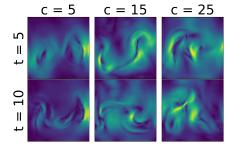
Figure 6: Outputs from DyAd while we vary encoder input but keep the forecaster input fixed. From left to right, the encoder is fed with flow with different buoyancy factor c=5,15,25. the forecaster network input has fixed buoyancy c=15.
