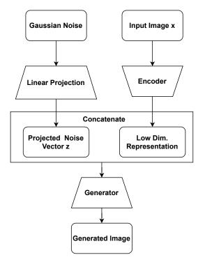
Figure S10: DAGAN Generator: The generator is composed of an encoder projecting the input image to a lower dimensional manifold. A random gaussian noise vector is transformed and concatenated with the bottleneck vector. The resulting vector is passed through the decoder (generator), which outputs the augmented image.
