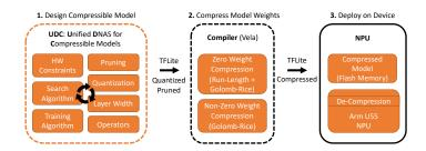
Figure 1: **Left:** NPU weight compression allows significant deployed model size reduction for TinyML. Compressed MBNetV2 size scales with increasingly aggressive quantization and pruning choices. **Right:** UDC designs compressible models, tailored to NPU deployment.
