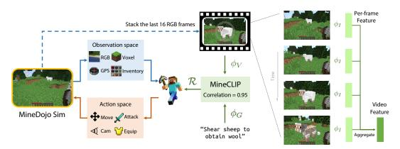
Figure 4: Algorithm design. MINECLIP is a contrastive video-language model pre-trained on MINEDOJO's massive Youtube database. It computes the correlation between an open-vocabulary language goal string and a 16-frame video snippet. The correlation score can be used as a learned dense reward function to train a strong multi-task RL agent.
