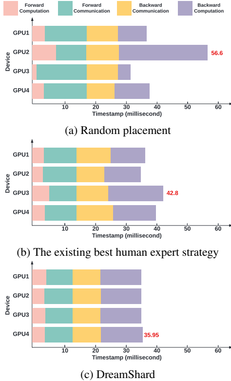
Figure 1: Visualization of random placement, the existing best human expert strategy, and DreamShard on a task of placing 50 tables on 4 GPUs. The dense computations and communications are omitted in the traces because they do not have an imbalance issue. We provide more visualizations in Appendix L.
