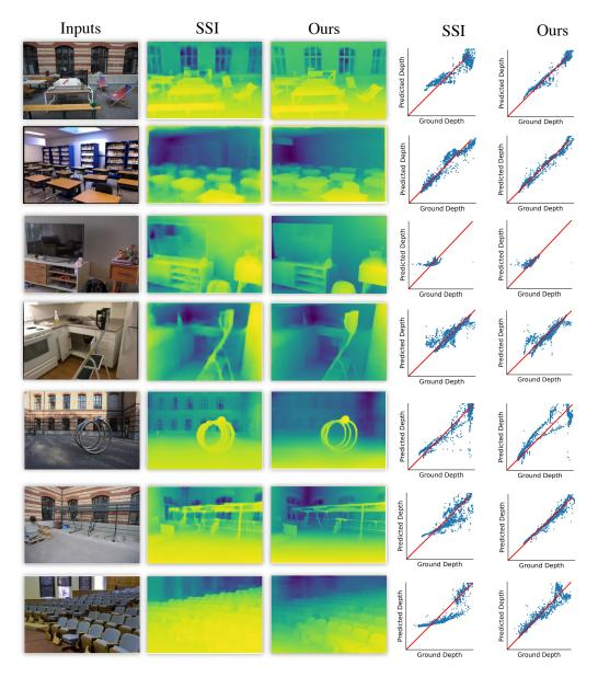
**Figure 4:** Qualitative comparison of our method and the baseline replying on instance-level normalization (SSI [24]). The red diagonal lines denote the ground-truth, and closer to it means better. Our method generates smoother surfaces, sharper edges and more details.
