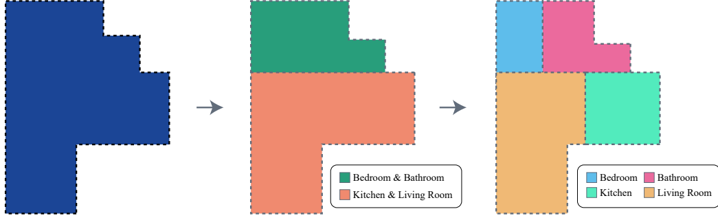
Figure 10: An example of the recursive floor plan generation algorithm, given an interior boundary and the room spec in Figure 7a. Here, we first divide the room into a “bedroom & bathroom” and a “kitchen & living room” zone. Then, within the “bedroom & bathroom” zone we place both the bedroom and bathroom, and within the “kitchen & living room” zone, we place both the kitchen and living room.
