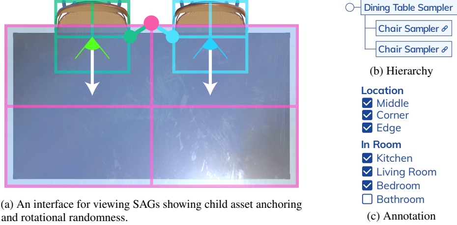
Figure 15: An example of a semantic asset group (SAG), where two chair samplers are parented to a dining table sampler. Both chairs are anchored to the top middle of the table.
