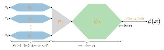
Figure 12: An illustration of the NestNet architecture realizing  $\phi = \phi_2 \circ \Phi_1 + f(\mathbf{0}) - \omega_f(\sqrt{d})$ . Here,  $\phi_1$  is implemented via Proposition B.1;  $\psi_1 : \mathbb{R}^d \to \mathbb{R}$  is an affine linear function;  $\psi_2$  is implemented via Proposition B.2.
