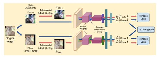
Figure 1: A Schematic representation of the proposed approach DAJAT
