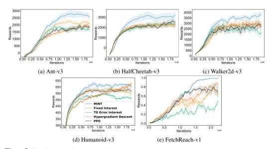
Figure 5: **Results on continuous control.** We compare MINT to various baselines including an emphatic variant of PPO using a fixed interest, as well as an interest based on the absolute value of the TD error. We also verify whether updating the learning rate via hypergradient descent can match the performance of MINT. Across environments, we notice that *adapting the interest via meta-gradients* is key to obtain consistent gains.
