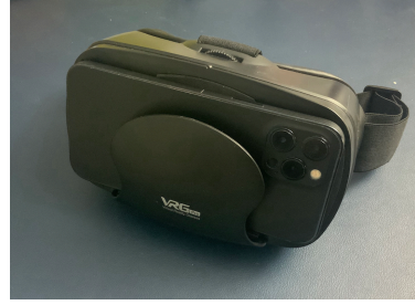
Figure 3: Our real-world dataset capturing equipment.
