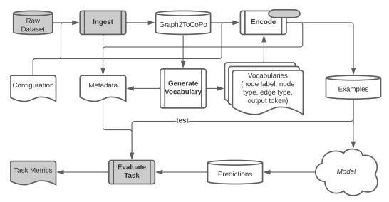
Figure 3: The software architecture of PLUR. The shaded components are task-specific. Everything else is common across all tasks.
