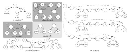
Figure 2: Representation alternatives for code2seq. The original AST is at the top left. Different arrow types represent distinct edge types.
