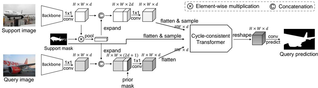
Figure 1: The network structure used in our experiments. The backbone network first extracts features for query and support images. To enable the pixel-wise comparison in transformer, the averaged foreground support feature is expanded and concatenated with both query and support features. Our Cycle-Consistent TRansformer (CyCTR) takes the flattened query and support features as well as the flattened support mask as input and produces the encoded query feature for prediction.
