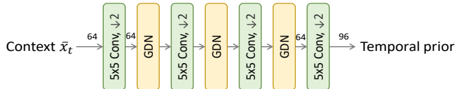
Figure 3: Network structure of temporal prior encoder network, same with the commonly used encoder in image compression [2] except the channel dimensions.
