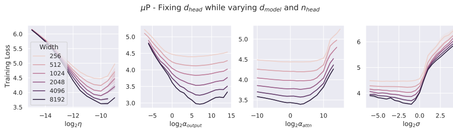
Figure 13: \mu\text{Transfer} across width when we fix d_{head} and vary d_{model} and n_{head} . \alpha_{output} , \alpha_{attn} are multipliers for output and key weights, and \sigma is initialization standard deviation.
