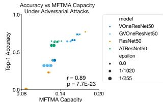
Figure SM3: MFTMA predicted capacity of class manifolds is well correlated with a model's performance under adversarial attack. Models include VOneResNet50 (blue), GVOneResNet50 (light blue), undefended ResNet50 (orange), and ATResNet50 (green) for clean images and PGD  $L_{\infty}$   $\epsilon = 1/1020$  and  $\epsilon = 1/255$  perturbed images.
