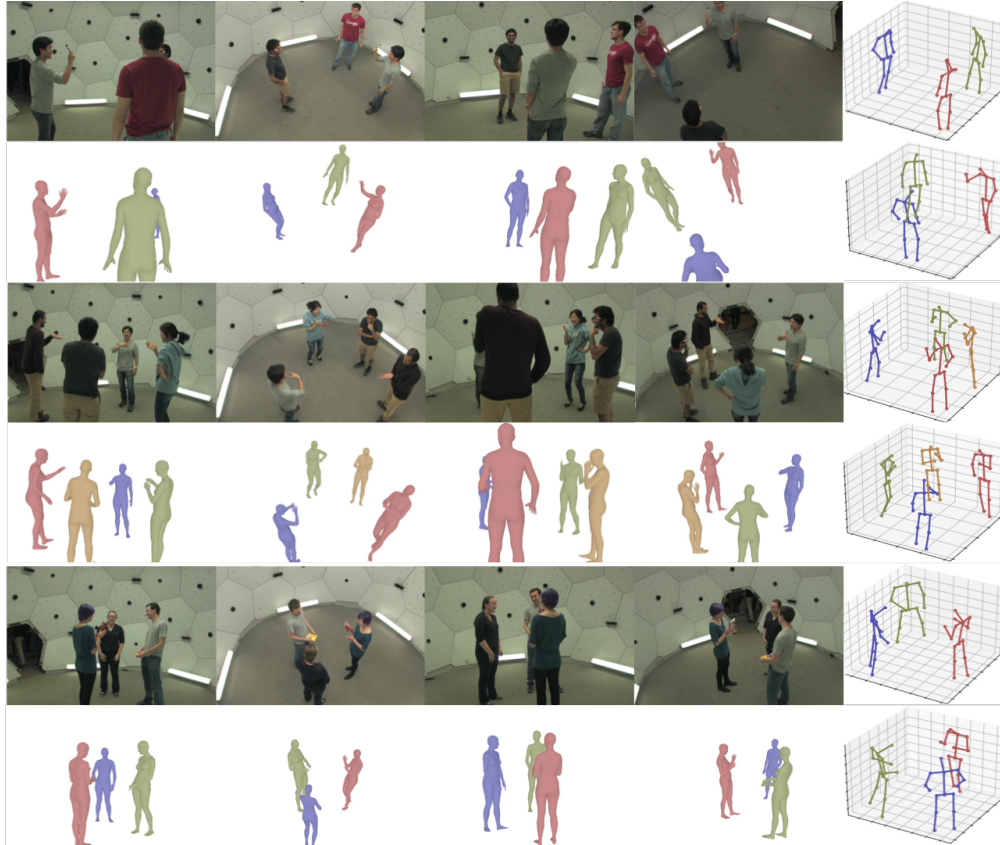
Figure S2: Example 3D pose estimations from Panoptic dataset. The left four columns show the multi-view inputs and the corresponding body mesh estimations from MvP. The rightmost column shows the estimated 3D poses from two different views. Best viewed in color.
