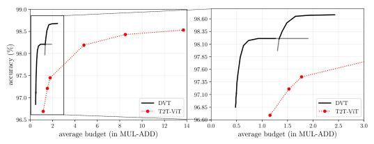
Figure 11: Top-1 accuracy v.s. GFLOPs on CIFAR-10. DVT is implemented on top of T2T-ViT-12/14.
