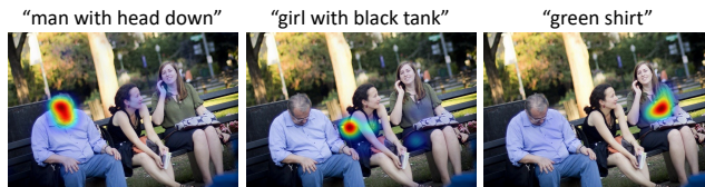
Figure 4: Grad-CAM visualization on the cross-attention maps in the 3rd layer of the multimodal encoder.
