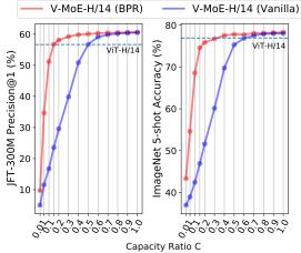
Figure 6: **Priority routing works where vanilla fails.** Performance vs. *inference* capacity ratio for a V-MoE-H/14 model with k = 2. Even for large C's BPR outperforms vanilla; at low C the difference is stark. BPR is competitive with dense by processing only 15-30% of the tokens.
