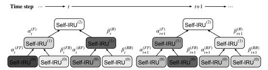
Figure 2: Soft depth gates  $\alpha_t^{(n)}$  and  $\beta_t^{(n)}$  for time step t and recursion node n (denoting F and R as the left child and the right child, respectively) control the extent of the Self-IRU recursion. The extent is indicated by greyscale of any node at the beginning of an arrow along an unrolled recursion path. These gates are between 0 and 1 and may vary across the temporal dimension, enabling dynamic soft recursion depth at each time step (here maximum depth L = 2).
