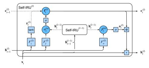
Figure 1: The self-instantiated recurrent unit (Self-IRU) model architecture. Circles represent gates that control information flow from dotted lines, and squares represent transformations or operators.
