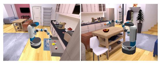
Figure 1: A mobile manipulator (Fetch robot) simulated in Habitat 2.0 performing rearrangement tasks in a ReplicaCAD apartment – (left) opening a drawer before picking up an item from it, and (right) placing an object into the bowl after navigating to the table. Best viewed in motion at https://aihabitat.org/docs/habitat2.
