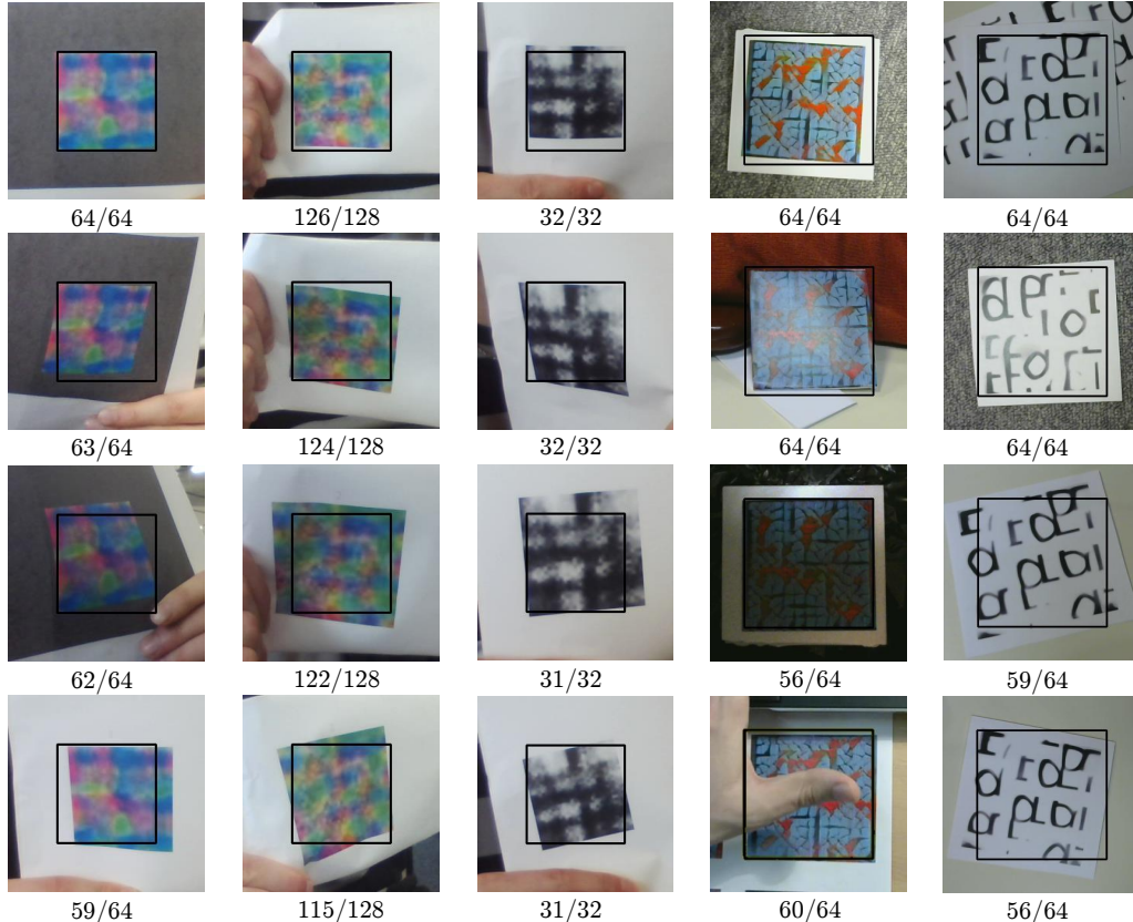
Figure 5: Screenshots of marker recognition process (black box is a part of the user interface and corresponds to perfect alignment). The captions are in (number of correctly recovered bits/total sequence length) format. The rightmost two columns correspond to stylized markers. These marker families were trained with spatial variances \sigma = 0.1, 0.05, 0.1, 0.05, 0.05 respectively. Larger \sigma leads to code recovery robustness with respect to affine transformation.
