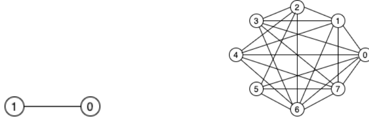
(a) Topology sparsity p_c = 0.8 with two nodes. (b) Topology sparsity p_c = 0.8 with eight nodes.
