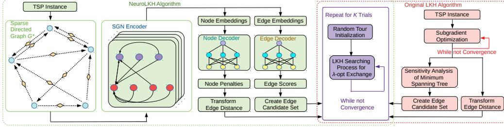
Figure 1: NeuroLKH algorithm and the original LKH algorithm.
