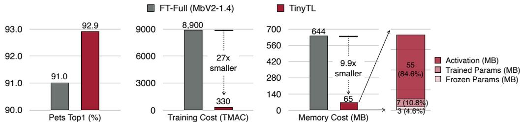
Figure 2: On-device training cost on Pets. TinyTL requires  $9.9\times$  smaller memory cost (assuming using the same batch size) and  $27\times$  smaller computation cost compared to fine-tuning the full MobileNetV2-1.4 [5] while having a better accuracy.
