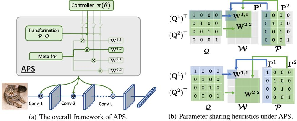
Figure 2: (a) The overall framework of the proposed affine parameter sharing (APS) for CNS. We take  $\mathcal{A} = \{1, 2\}$  for illustration; (b) A 2-dimensional illustration of affine parameter sharing with ordinal selection (up) and independent selection (down). The candidate kernel is constructed by transforming the meta-weights into proper shapes with two transformation matrices.
