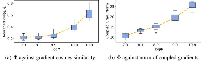
Figure 3: The variation of  $\Phi$  against the cosine similarity (left) and the norm of coupled gradients (right). We take the training of a 20-layer residual network for demonstration.
