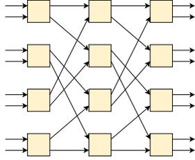
Figure 1: Shuffle-Exchange network.
