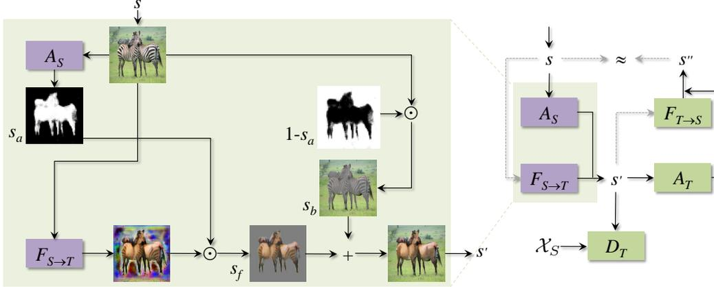
Figure 2: Data-flow diagram from the source domain  $S$  to the target domain  $T$  during training. The roles of  $S$  and  $T$  are symmetric in our network, so that data also flows in the opposite direction  $T \rightarrow S$ .
