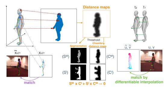
Figure 2: **Differentiable rendering** of body joints (left), segmentation (middle) and mesh vertex motion (right).
