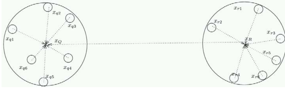
Figure 1: The basic idea is to approximate the kernel sum contribution of some subset of the reference points X_R , lying in some compact region of space R with centroid x_R , to a query point. In more efficient schemes a query region is considered, i.e. the approximate contribution is made to an entire subset of the query points X_Q lying in some region of space Q , with centroid x_Q .
