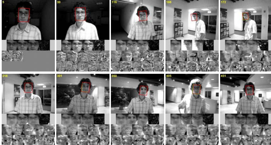
Figure 1: A person moves from dark toward bright area with large lighting and pose changes. The images in the second row shows the current sample mean, tracked region, reconstructed image, and the reconstruction error respectively. The third and forth rows shows 10 largest eigenbases.
